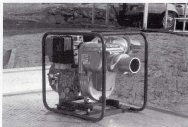
Honda diesel provides loads of power to 4" Aussie pump
